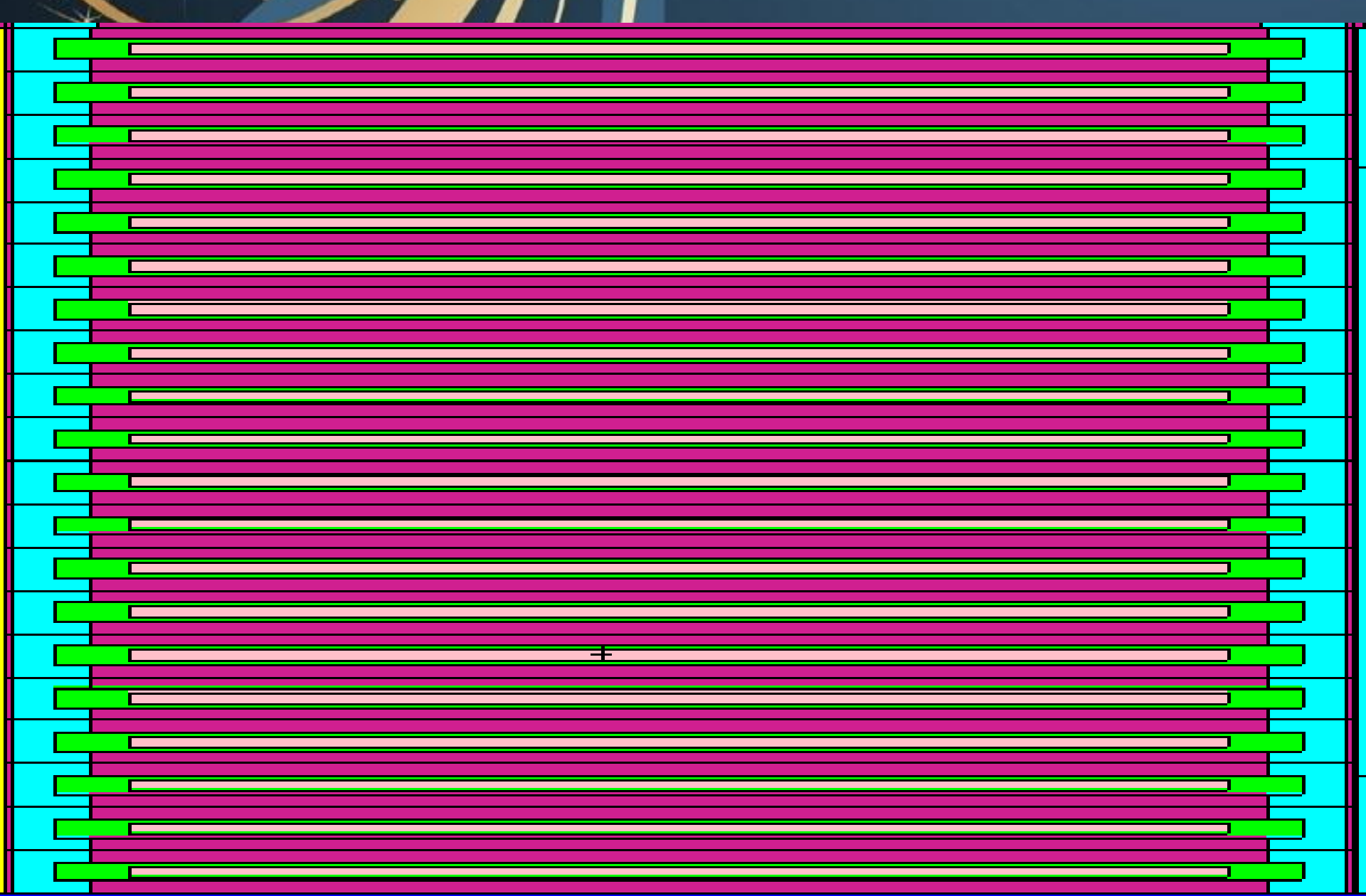
Fig. (4.a) Standard LEU Fuel Element (20 plates )
