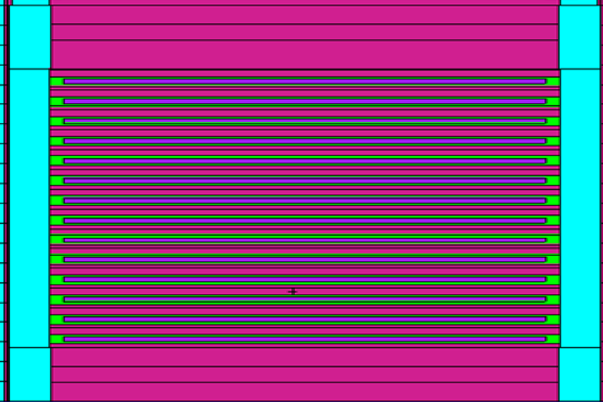
FIG (4.b) Control (LEU) Fuel Elements 14 Plates
