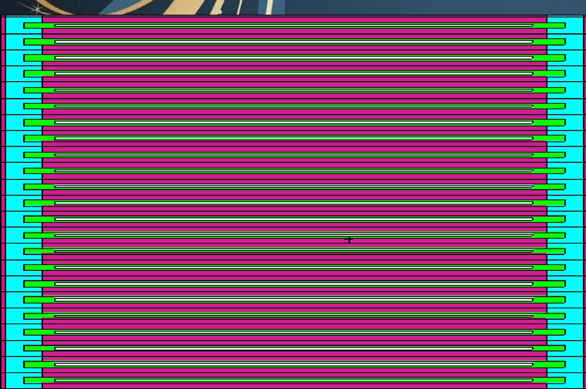
FIG.(3.a) Standard HEU Fuel Element (23 Plates)
